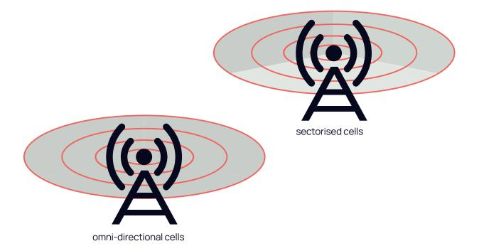
A sectorised site employs directional antennas, which limit transmission of each radio channel to a specific part of the base station coverage area. Sectorised sites can be configured in a variety of ways, but typically have either three or six sectors.
